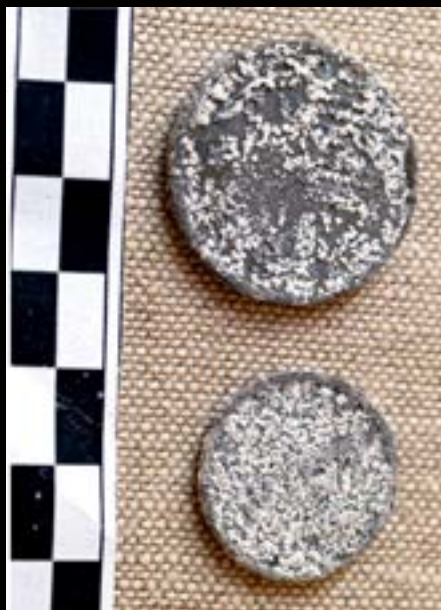
Fig. 1. Coins of denominations of 5 and 10 marks from the Łódź ghetto made of magnesium alloy, before preservation works (photo by M. Kołyszko)
